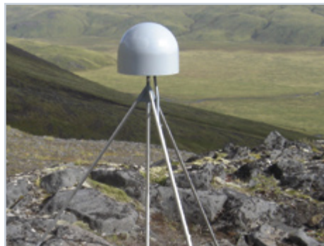
Trimble GNSS Choke Ring Antenna
