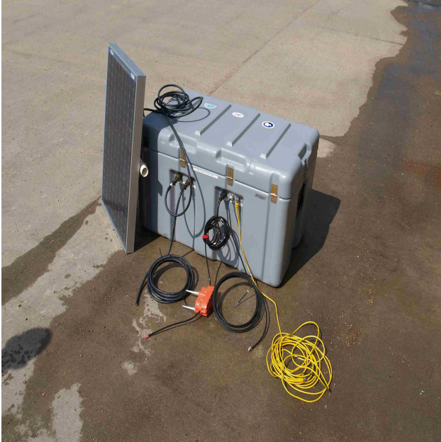
Complete power/enclosure/GPS system provided
