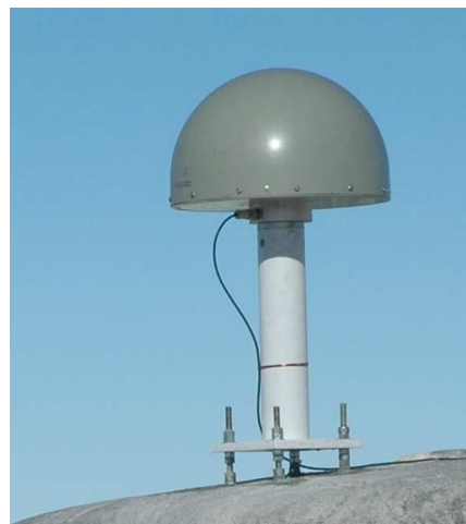
Low profile forced centering GPS mast 16.8" version Installed with 0.5" x 12" expansion bolts
