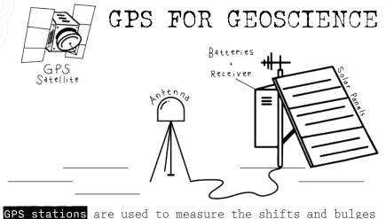
**GPS stations** are used to measure the shifts and bulges of our planet using the same technology as your cell phone. However, they are far more precise, allowing us to measure ground movement as slow as a millimeter (0.04 inches) per year by recording positions day after day and year after year.
