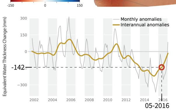
NASA's GRACE (Gravity Recovery and Climate Experiment) mission is actually a pair of satellites that fly in formation, precisely measuring the spacing between them. Earth's gravitational pull is not uniform because of variations in the mass of material-whether bedrock or water or glacial ice-below you in any given location. These variations cause the satellites to speed up or slow down ever so slightly, temporarily increasing or decreasing the spacing between the pair.
