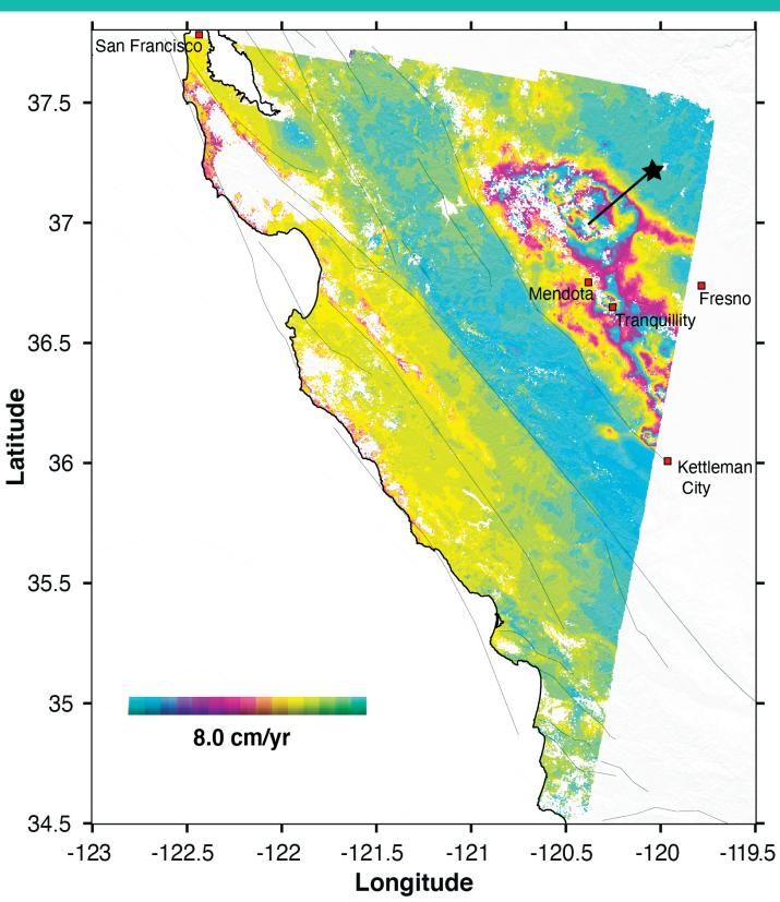
InSAR stands for "Interferometric Synthetic Aperture Radar." Satellites bounce radar signals off the surface of the Earth and use the delay in the signal's return to measure distance extremely precisely. This technique produces a high-resolution 3D map of the surface that shows every hill and valley. By comparing all the 3D maps made by multiple passes of a satellite, like the European Space Agency's Sentinel-1A satellite shown here, we can see if anything has moved or changed shape.
