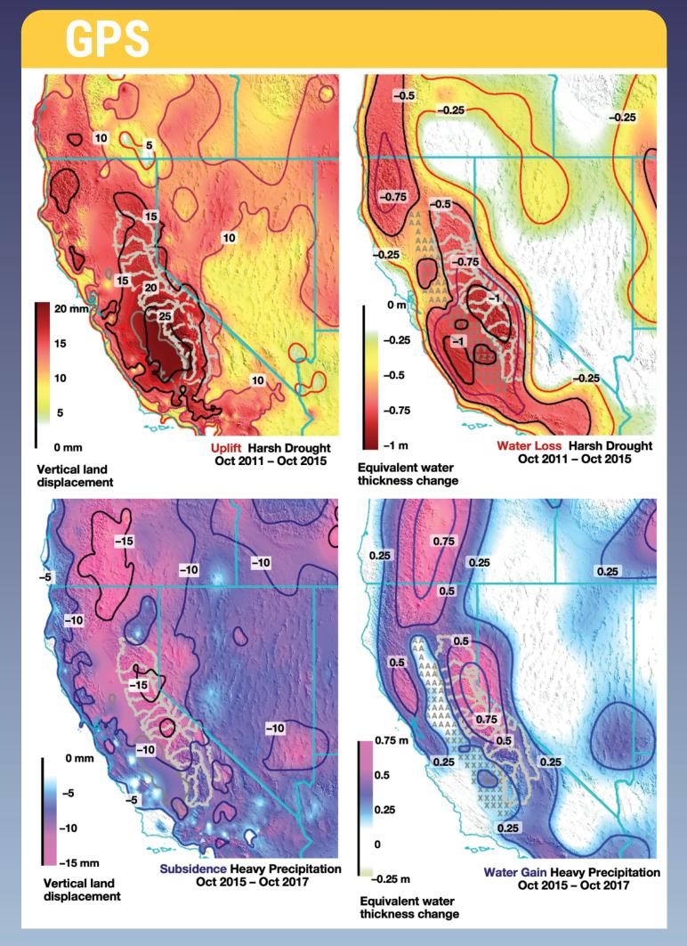
High-precision Global Positioning System stations can measure location far more exactly than your phone. As the ground beneath them moves, they are sensitive enough to detect changes of less than 1 millimeter per year! They measure vertical movement in addition to horizontal, which means they can also monitor groundwater.
