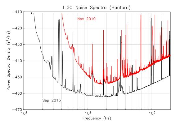
The decrease in instrument noise level from 2010 to 2015 was what made the observation possible.
