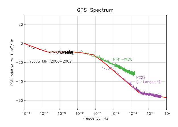
Piecewise linear approximation to noise spectrum, using a range of datasets/analyses.
