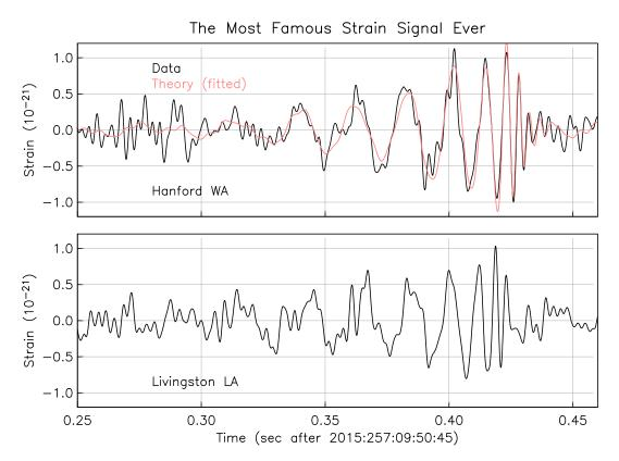
Data from two *really good* laser strainmeters (LIGO), showing deformations of the space-time continuum by gravitational radiation from two black holes that "inspiraled" and merged during the early Neoproterozoic.
