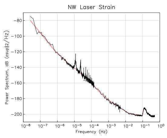
We use a high-quality strain record, from the NW-SE laser strainmeter at Piñon Flat Observatory, and fit a spectrum to this that consists of linear segments (in log-log space: a composite power-law spectrum).
