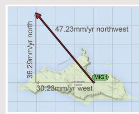
Each arrow originates at a GPS station, and points in the direction the station is moving. Its length is proportional to the station's speed, or velocity. The faster the station is moving, the longer the arrow. The scale for the arrows is given at the bottom of the map. Station motions are given in millimeters per year. That's tiny—but even small motions can tell us a lot about the Earth.
