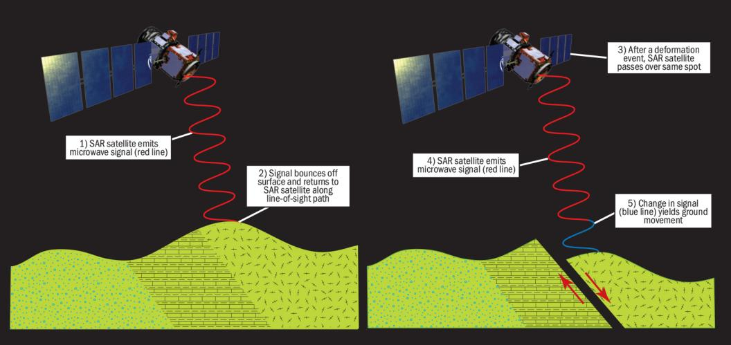
Different SAR satellites emit different microwave wavelengths, providing different levels of detail.
