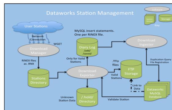
These modules download files from GNSS receivers (that have internet connections), temporarily storing the files in a local station/data directory, ingesting file information into the Dataworks database, and storing files on a local ftp server for distribution. Ingest and export for data acquisition by other means (e.g. manual download) can also be handled.
