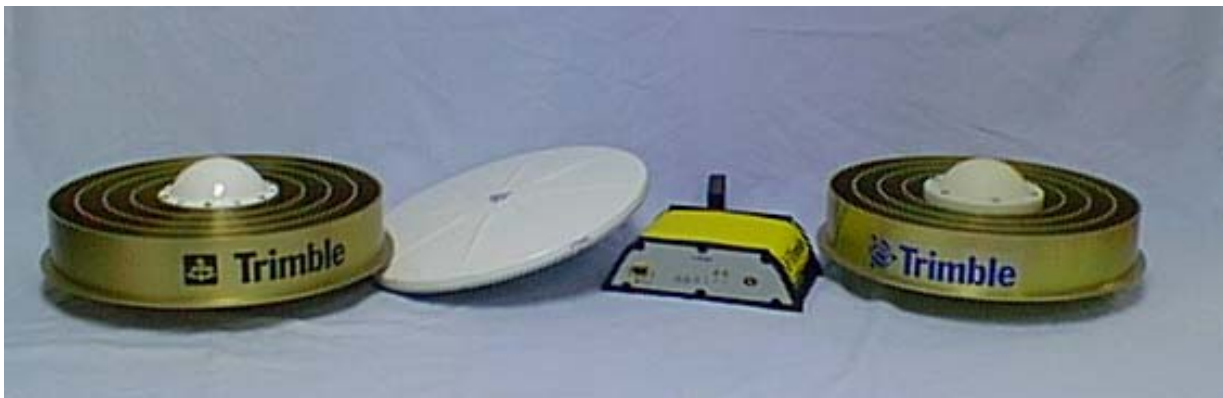
Figure 2.5 - Pictured above from left to right: TRM 29659 DM Choke, TRM 41249 Geod, NetRS (GPS Receiver), and the TRM 49700 Choke.
