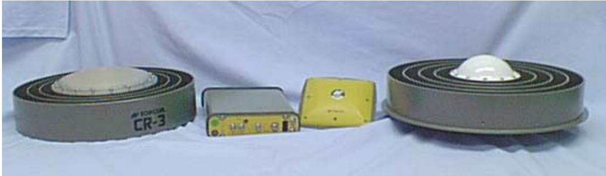
Figure 2.4 – Pictured above from left to right: TPS CR3 Choke, Odyssey RS (GPS receiver), TPS PG-A1 Geod, and TPS CR4 DM Choke.
