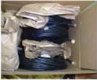
Topcon Antenna Cables
