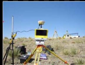
Figure 5. TLS unit with gray skirt base showing RTK-GPS and antenna.
