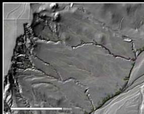
Figure 3. West Bijou Creek Airborne LiDAR image, gullies are represented by green circles and were measured in ArcGIS. Gullying in the area of this area started after the 1982 flood.
