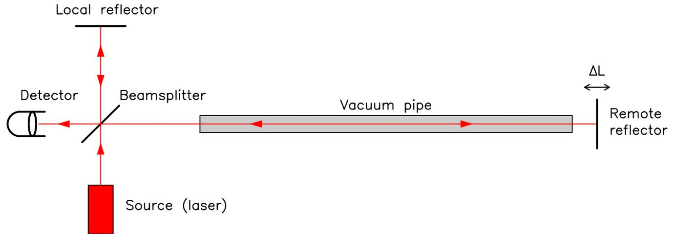
A **Michelson interferometer** has two arms, one fixed (to the local reflector) and one variable (to the remote reflector).
