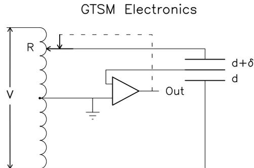
An input voltage is divided in a ratio transformer, with the output (ratio to input good to 7 figures) applied to the capacitor plates. The ratio  $R$  is varied both to minimize the output from the center plate, and also to calibrate the system.
