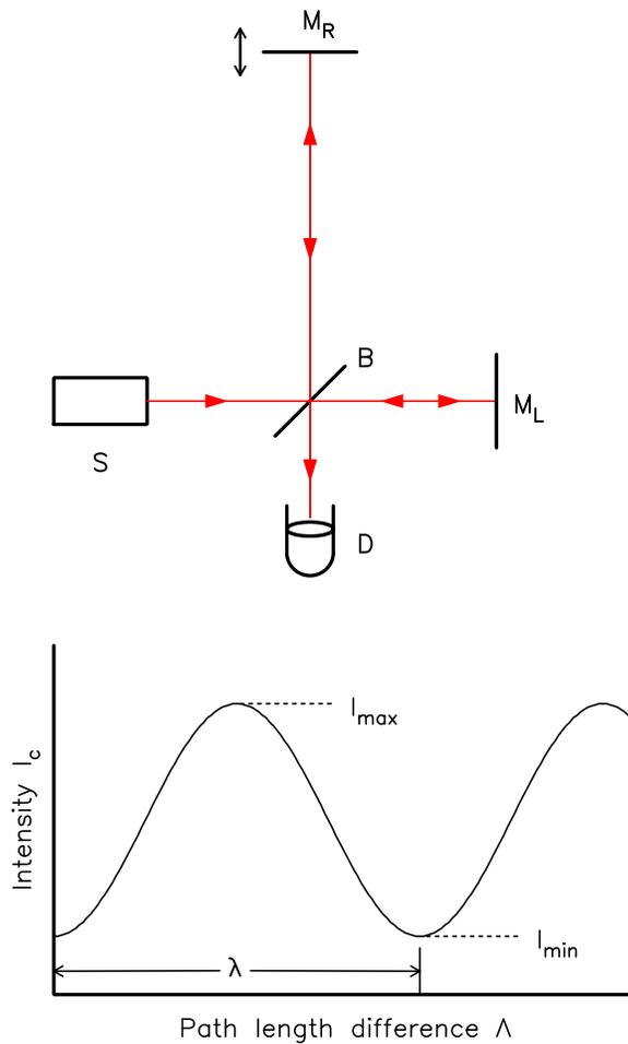
A **Michelson interferometer** has two arms, one fixed (to  $M_L$ ) and one variable (to  $M_R$ ).
