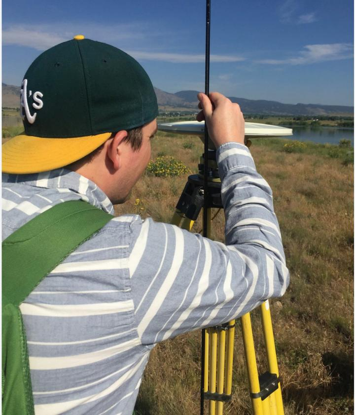
hchpad intern Bradley Norman and UNAVCO polar engineer Annie Zaino set up the base station for a GPS survey of the St. Mary's glacier near Idaho Springs, Colorado.
