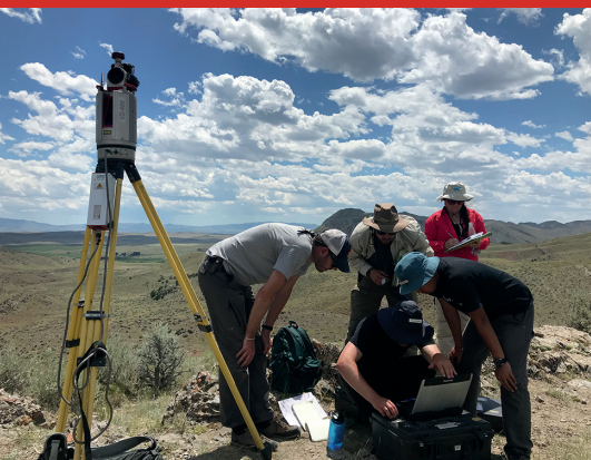
Students from the Indiana University Geologic Field Station use a ground-based lidar system to scan geological structures in southwest Montana.
