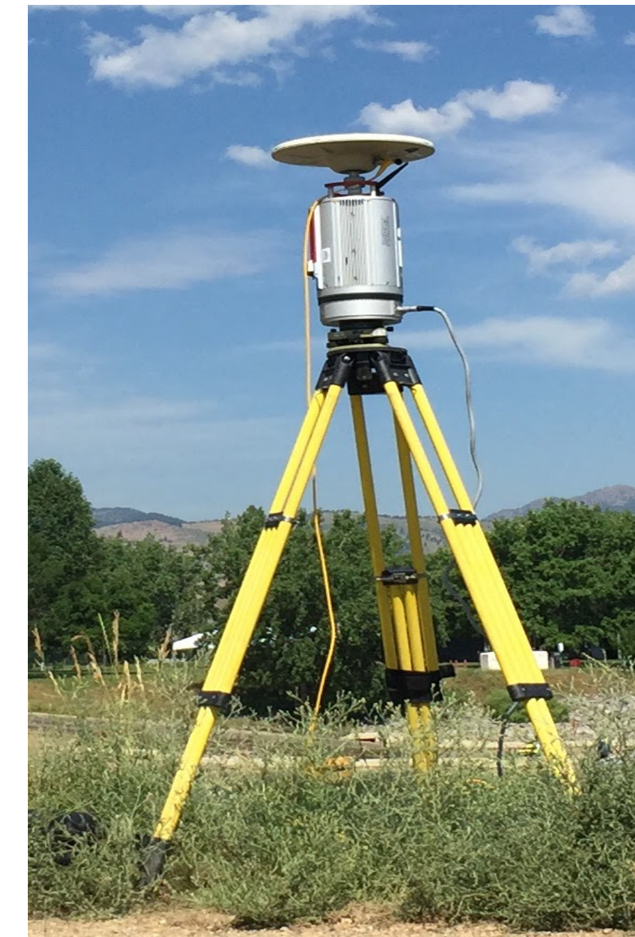
Figure 1: The RIEGL VZ-400 terrestrial laser scanner with the Zephyr Geodetic antenna mounted on top.
