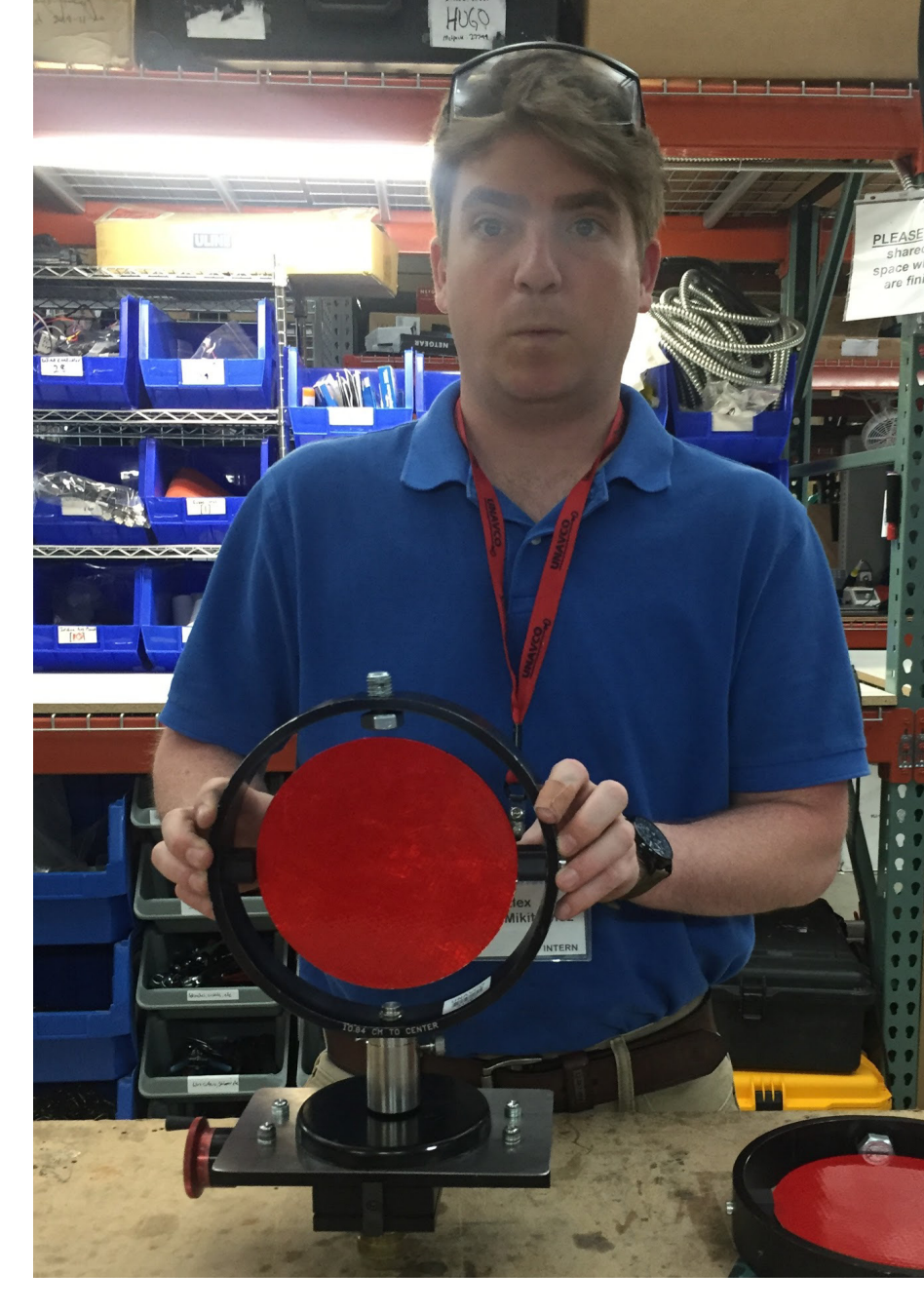
Figure 2: Alex Olsen-Mikitowicz displays the target mounted to the lateral translation bar.
