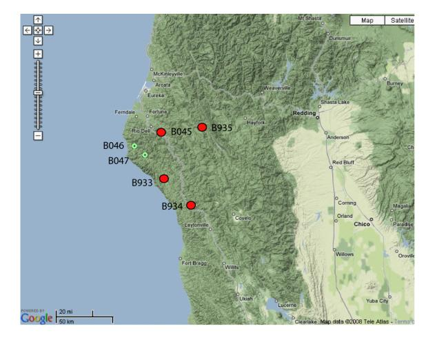
Mendocino PBO strainmeters, October, 2008. Green dots represent boreholes that only have a seismometer.
