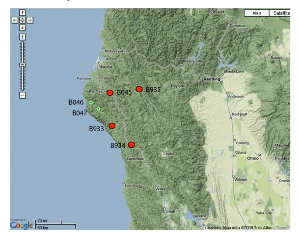
Mendocino PBO strainmeters, October, 2008. Green dots represent boreholes that only have a seismometer.
