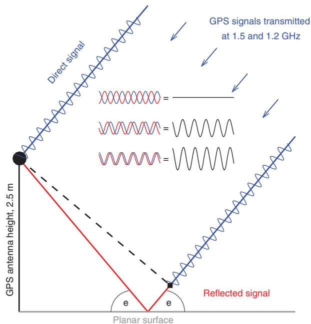
**FIGURE 1** | Multipath geometry for a horizontal planar reflector. Satellite elevation angle is designated by the variable  $e$ . A GPS antenna measures the interference between the direct (blue) and reflected (red) signals. Examples of this interference are shown in the inset.
