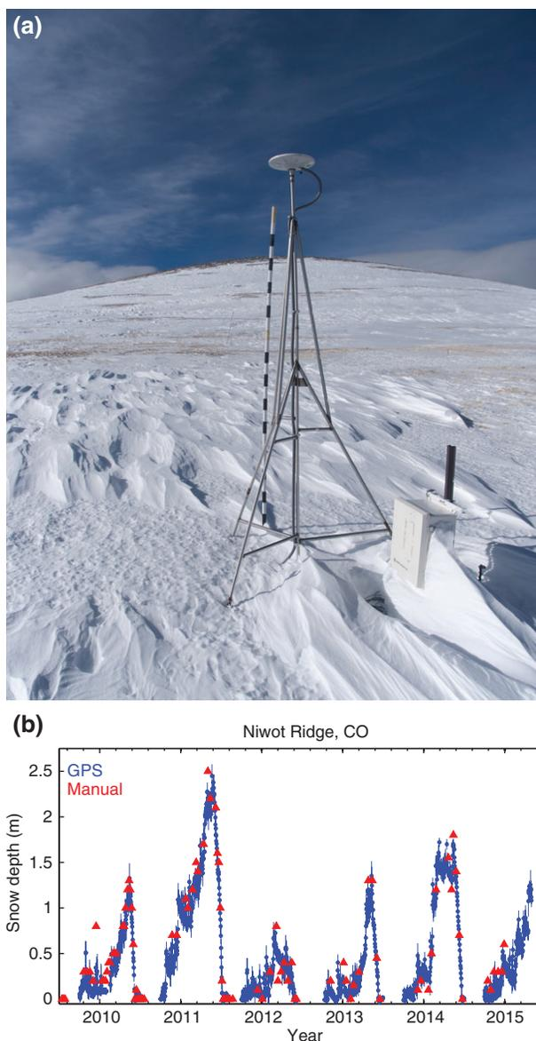
**FIGURE 5** | (a) Photo of the Niwot Ridge GPS antenna. Snow depth is also measured at the black and white pole by the Niwot Ridge Long-Term Ecological Research group at 2-week intervals during the snow season. (b) Snow depth measured by GPS-IR (blue) and at the pole shown in panel (a) photograph (red).
