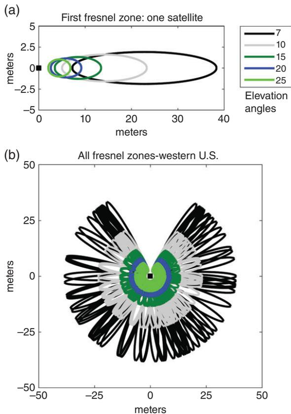
**FIGURE 2** | (a) The first Fresnel zone for a single satellite track is depicted for satellite elevation angles of 7, 10, 15, 20, and 25 degrees and an antenna height of 1.8 m. (b) Map view for the GPS-IR footprint in the western United States for all transmitting GPS satellites. The location of the GPS antenna is shown as the black square.
