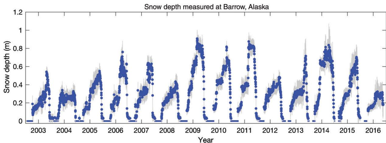
**FIGURE 7** | GPS-IR measurements of snow depth at Barrow, AK (Plate Boundary Observatory site SG27). To improve clarity of the snow depth estimate in blue, one standard deviation error bars are shown in gray.
