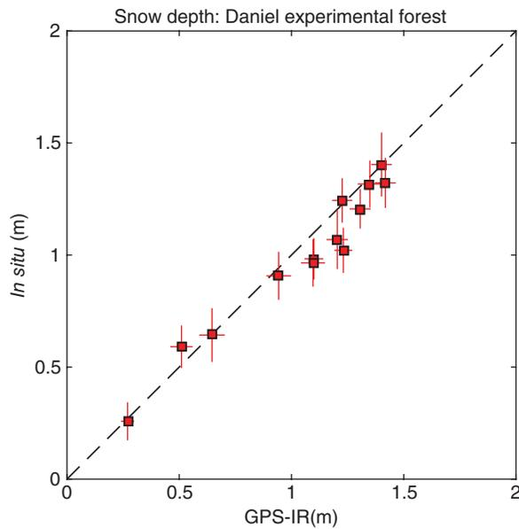
**FIGURE 6** | Utah State Daniel Experimental Forest comparison between GPS-IR and *in situ* hand measurements measured in the GPS-IR footprint.
