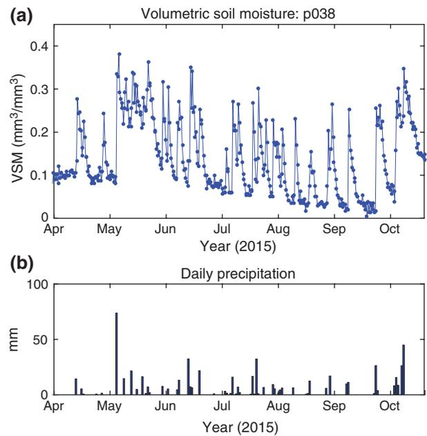
**FIGURE 8** | (a) Volumetric soil moisture (VSM) estimated using GPS-IR for Plate Boundary Observatory site P038, located in eastern New Mexico. Soil moisture is estimated twice per day at this site. (b) Daily precipitation is measured with a Vaisala WXT520 sensor.
