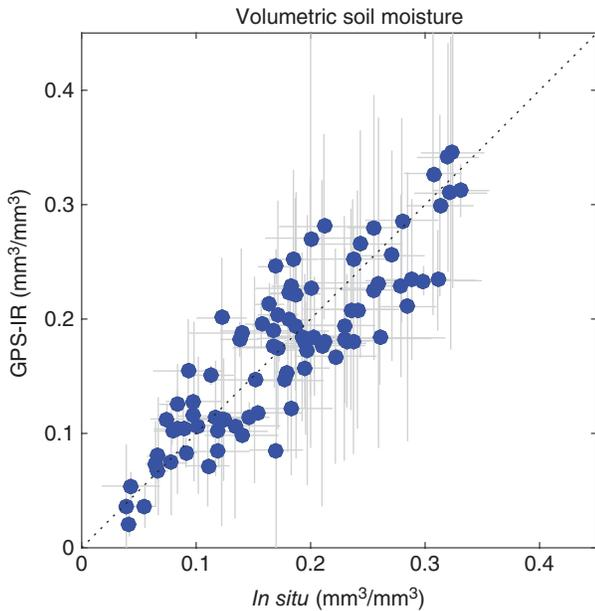
**FIGURE 9** | Comparison between *in situ* soil moisture probes and GPS-IR. Error bars represent one standard deviation. Root mean square error is 0.039 mm<sup>3</sup>/mm<sup>3</sup>.
