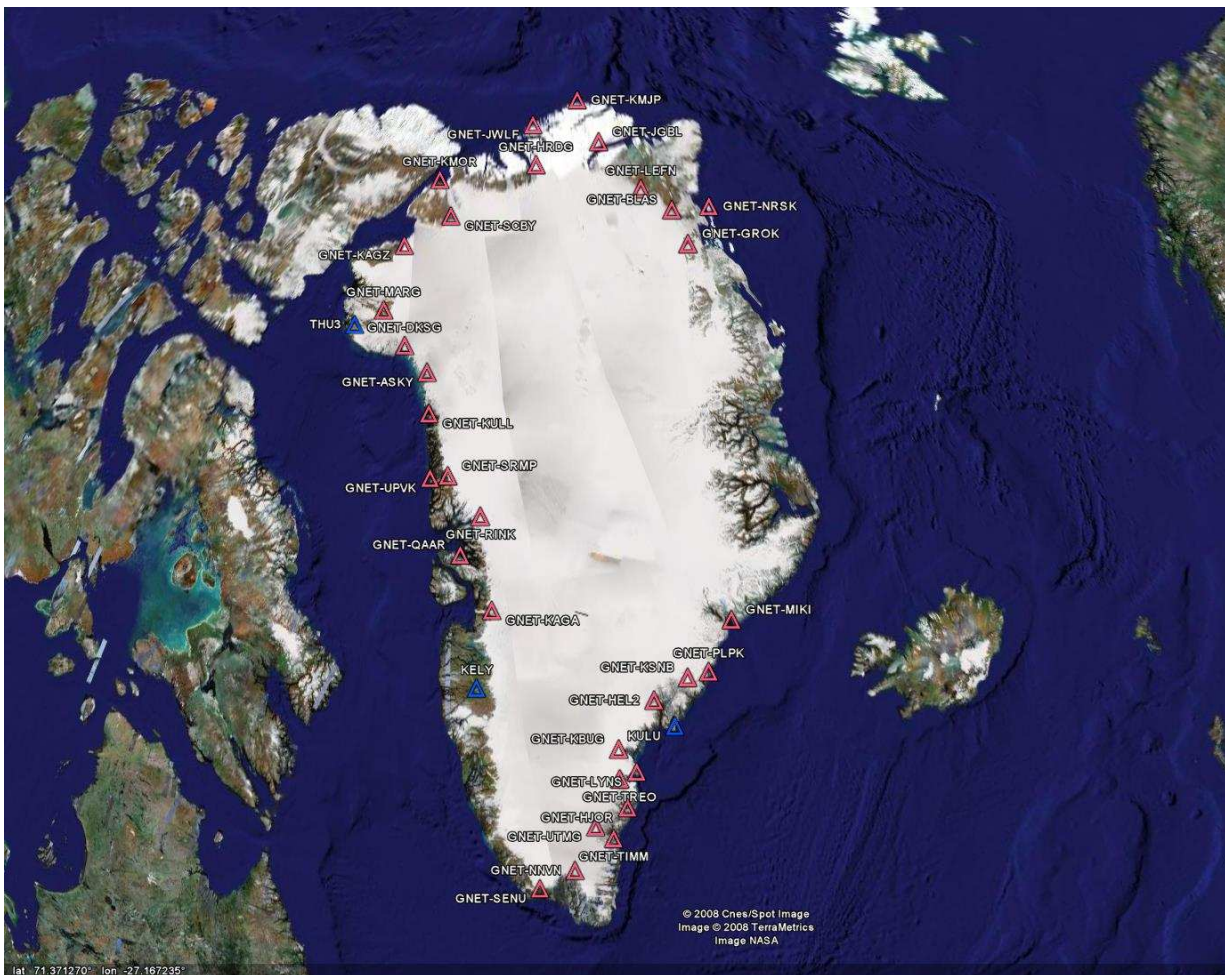
Figure 8 – Construction of the POLENET/GNET GPS network continued in 2008, with stations added in the north and southwest. When completed GNET will provide bedrock GPS sites around the entire circumference of Greenland.
