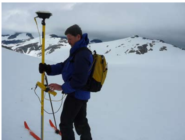
Figure 11 - Scott McGee, JIRP's head surveyor, measures the position of a point on the Lemon Glacier.
