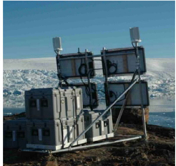
Figure 6 (left) – Installation of an MRI system field kit on Mt. Erebus, Antarctica, with GPS and met sensors.
