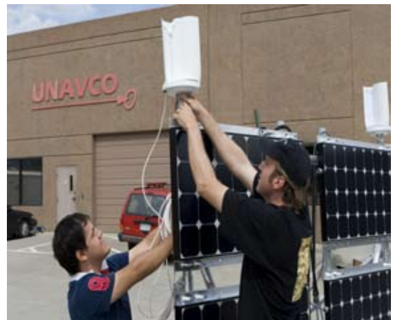
Figure 3 - Ezer Patlan with UNAVCO polar engineer and project mentor Seth White working on a polar remote power and communication system.
