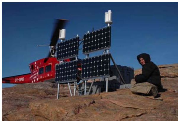
Figure 13 - Field engineer Marianne Okal at Doecker Smith Gletscher site DSGK. The system is powered by four 90W solar panels and two Forgen 500 wind turbines. For year-round continuous operation.
