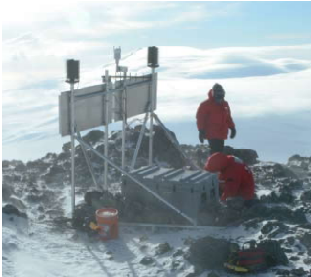
Figure 6 (left) – Installation of an MRI system field kit on Mt. Erebus, Antarctica, with GPS and met sensors.
