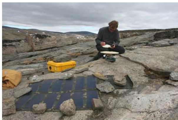
Figure 14 - UNAVCO engineer Seth White sets up GPS base receiver at Green Valley solifluction site, near Thule, Greenland.
