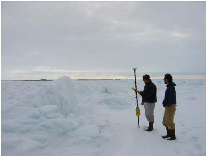
Figure 3 – RTK survey equipment on the Chukchi Sea ice.
