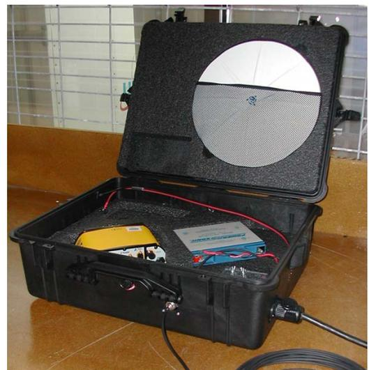
Figure 6: NetRS custom package developed at UNAVCO before the 2004/05 field season.
