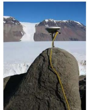
Figure 8: A Zephyr antenna is used to measure surface flow in Taylor valley.
