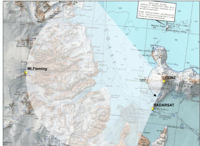
Figure 5b: Extent of radio communications from the repeater site at Truncated Cones.
