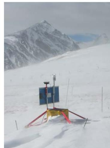
Figure 4: Testing a weather station integrated with the GPS receiver at the Niwot Ridge test facility.
