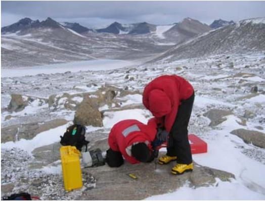
Figure 11: Anne Benninger (RPSC) and Beth Bartel (UNAVCO) drill a hole for a new survey marker near Clark glacier.
