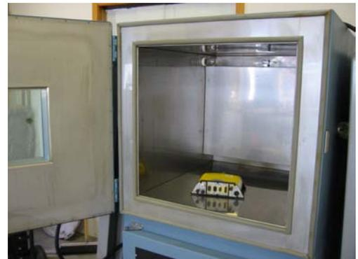
Figure 3: Environmental test chamber recently acquired by UNAVCO.
