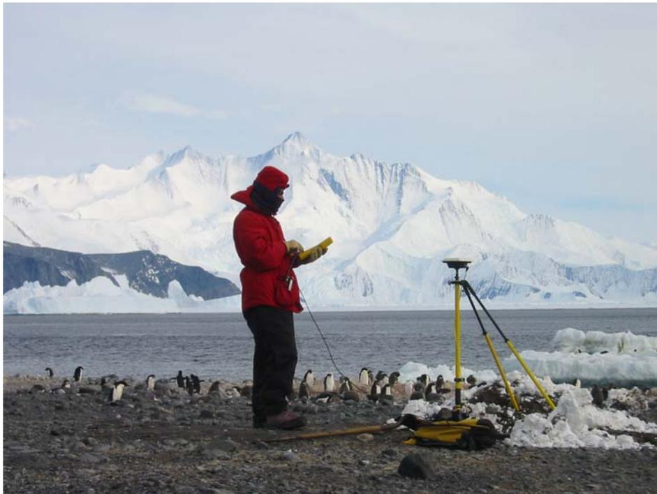
Figure 3: Surveying precise ground water heights at Cape Hallett.
