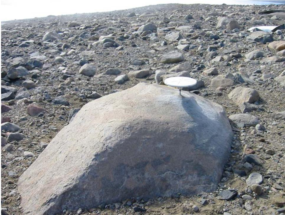
Figure 5: Base station for Commonwealth Glacier spreading rate survey, B-042-F.
