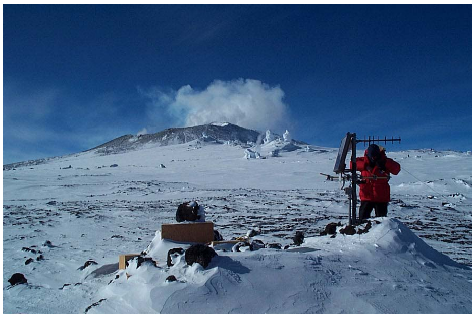
Figure 1 – Continuous GPS and seismic station CONZ on Mount Erebus
