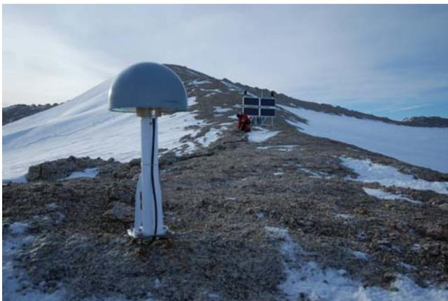
**Figure 6.** The most recent POLENET installation in the extremely remote and inaccessible Marie Byrd Land. The 1-m mast GPS monument used for most POLENET remote stations was designed at the Ohio State University for rapid installation in exposed bedrock.
