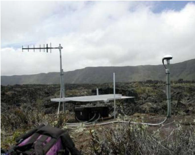
Figure 2-1. Single frequency GPS station (GV06) in the Sierra Negra Caldera, installed in June 2002 (Dennis Geist, PI).
