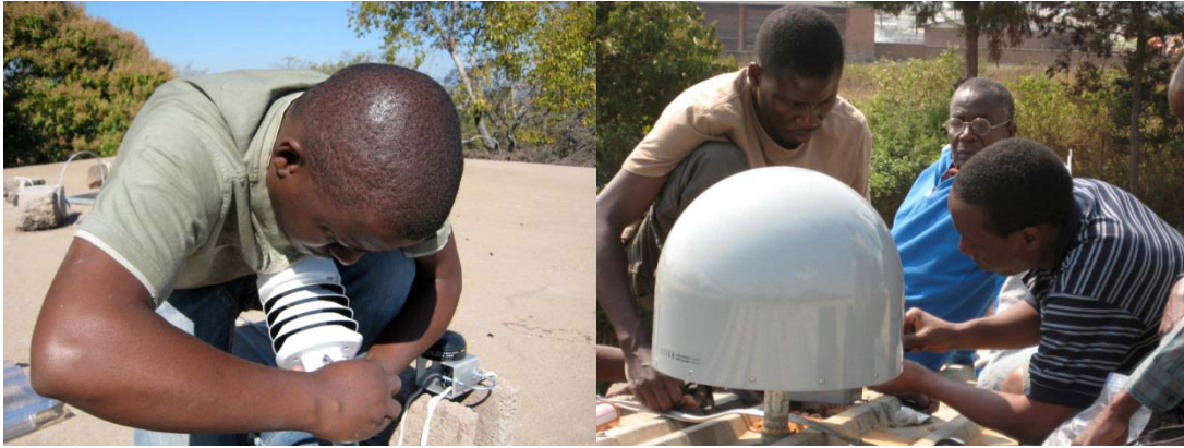
Figure 4. Left - Robert Kometsi installs the meteorological sensor on top of the seismic vault at Itexi-Tezi, Zamiba. Right - Winstone Kapanje (left), a local collaborator with the Geologic Survey of Malawi in Zomba, Fred Tugume, and others help to install the GPS antenna on the roof of the Survey office building.
