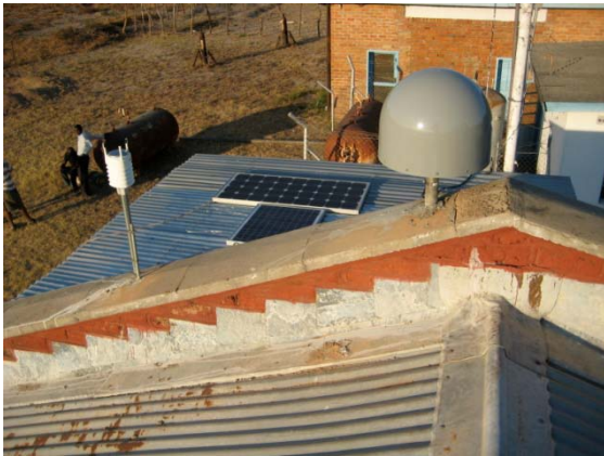
Figure 3. The GPS station with meteorological sensor in Mongu, Zambia. The equipment is installed on the roof of the Zambian National Meteorological Survey.
