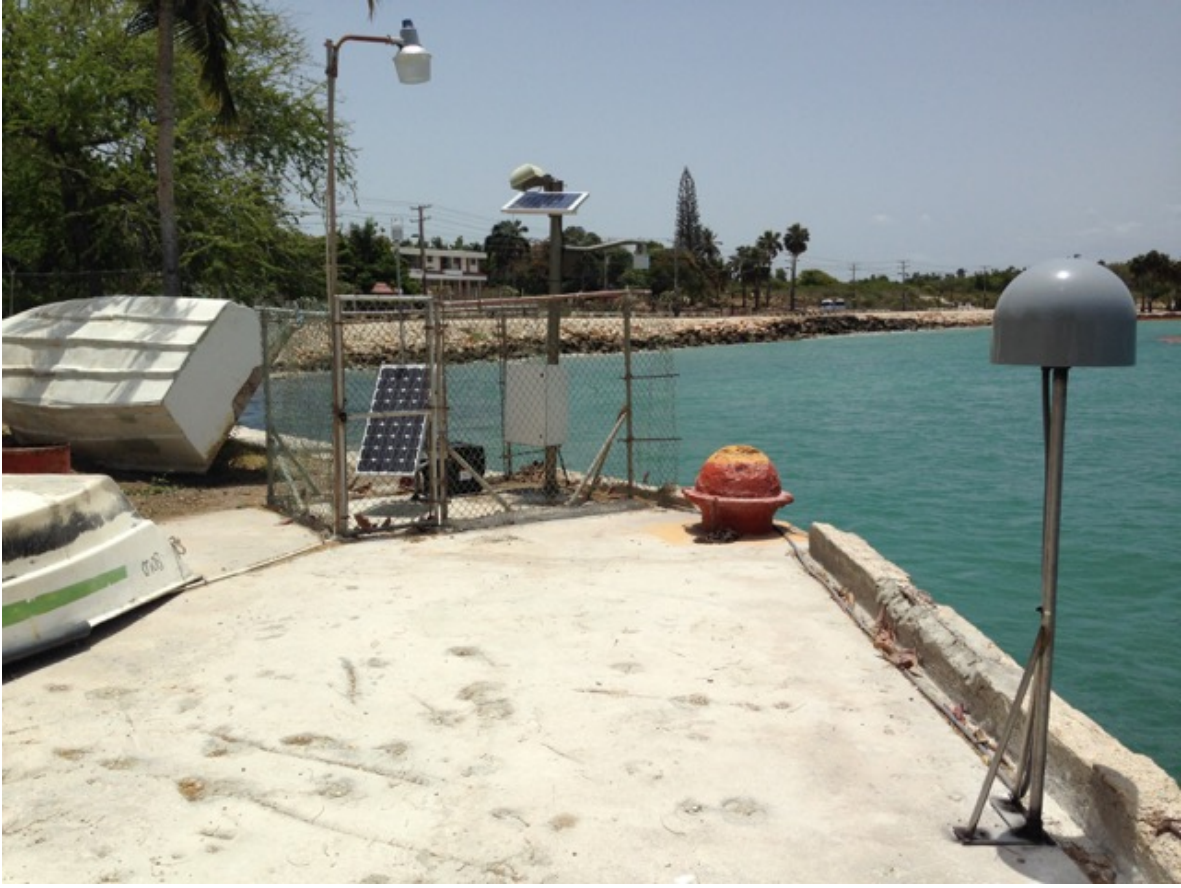
Figure 8. Overview of TGDR cGPS station co-located with tide gauge.
