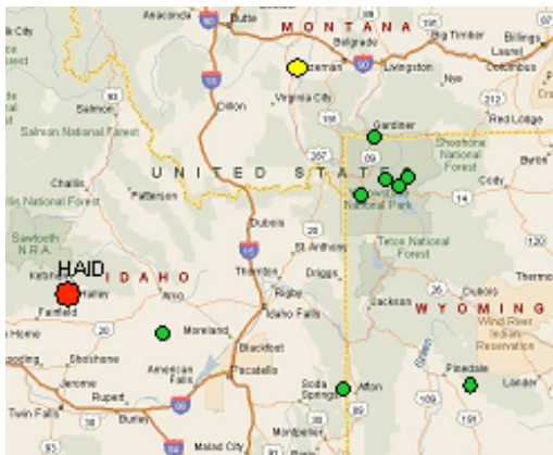
Figure 2–3. Graphical view of station operations. Red = no data in last 5 days, yellow = no data in last 2 days, green = data current. Station symbols are hyperlinked to plots of data availability, quality and station metadata.
