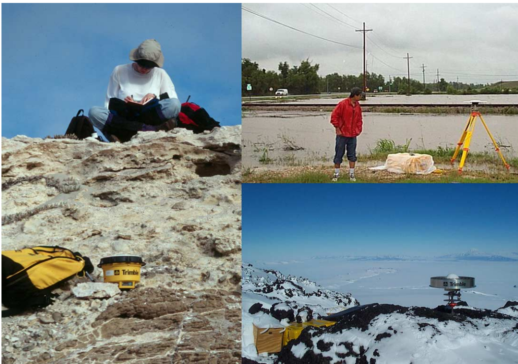
Figure 1-1. Rapid static survey of raised marine terraces to measure fault-related folding in California's Northern Channel Islands (left); vertical control benchmark for the Mississippi Delta project used to document Holocene sea-level change (upper right); Mt. Erebus, Antarctica volcano deformation campaign network site at Hooper's Shoulder (lower right).
