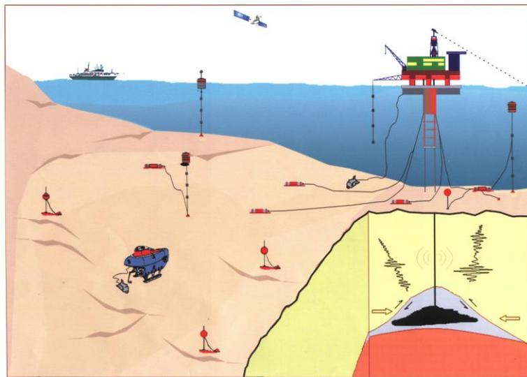
Figure 1. A general structure of the coastal zone geophysical hazard observation system based on drilling platforms
