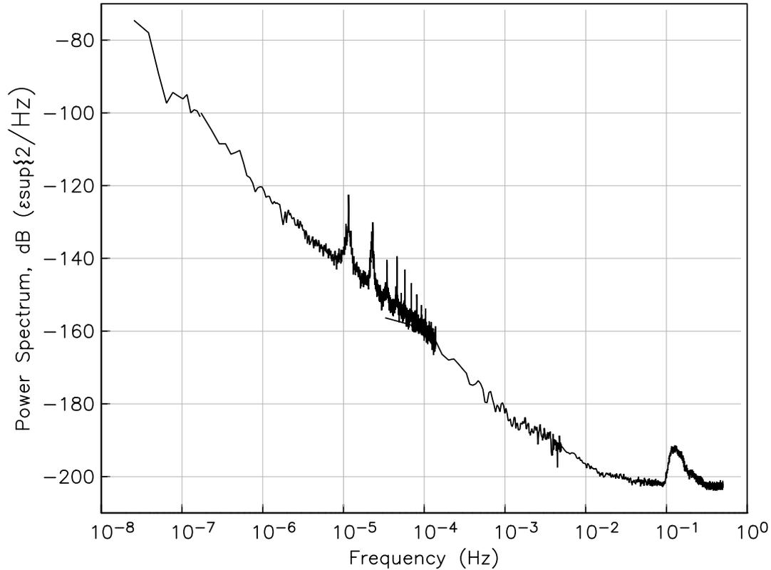
We use a high-quality strain record, from the NW-SE laser strainmeter at Piñon Flat Observatory:
