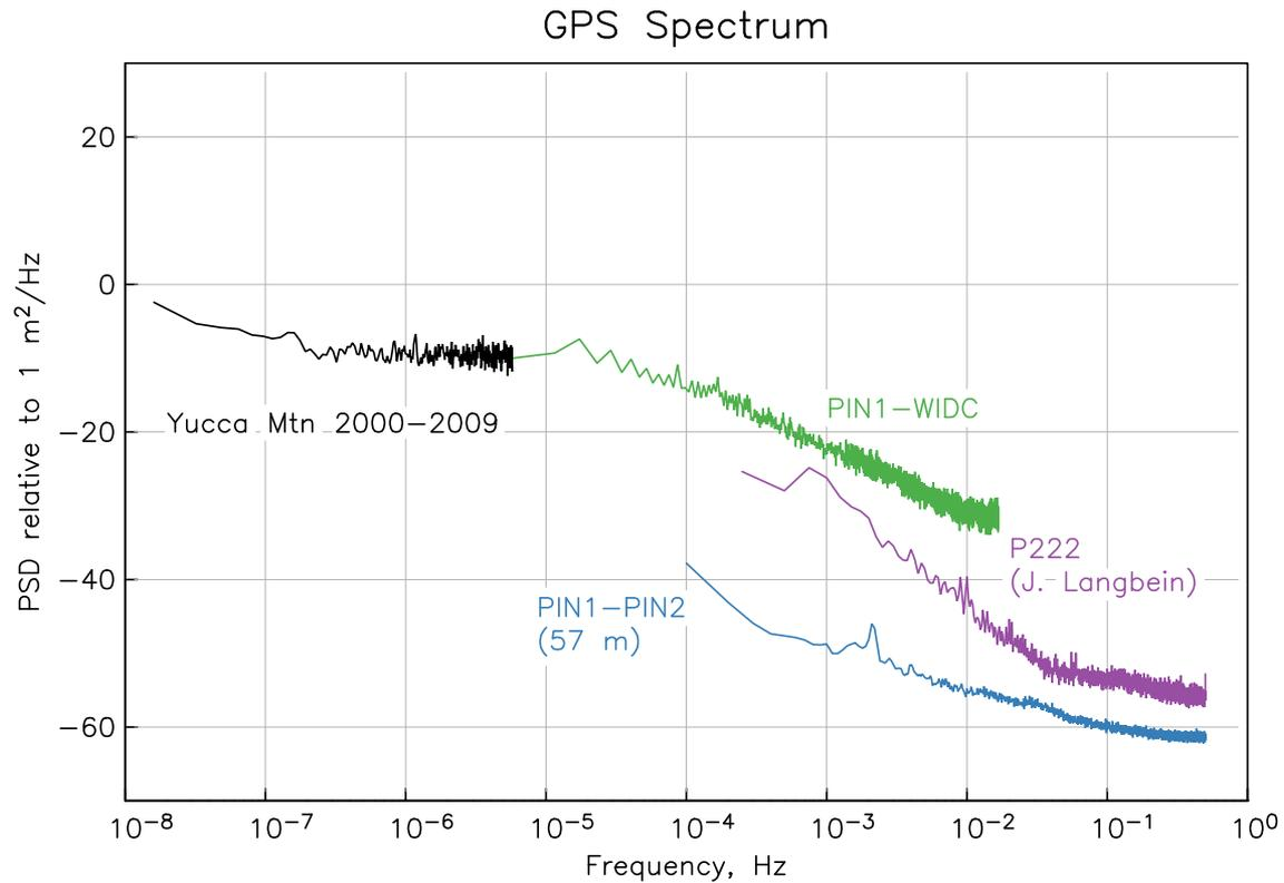
PIN1-PIN2 is a very short baseline – note that noise floor close to -60 db (1 mm rms white noise).
