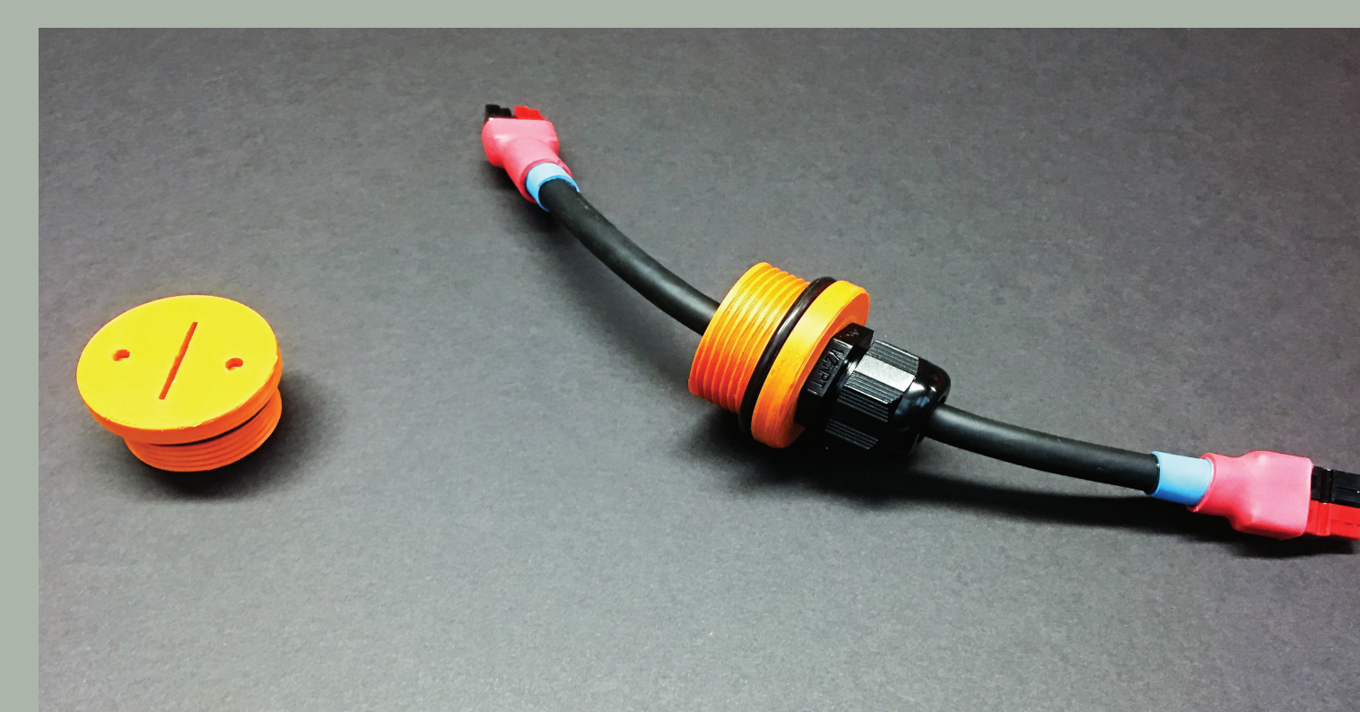
Figure 19: Left, one of the basic caps printed for the campaign boxes. Right, a cap with power connections designed to interface with solar panels.
