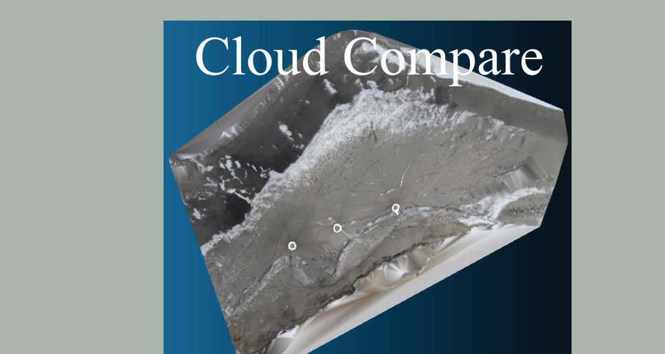
Figure 11: Mesh has been applied to the point cloud in CloudCompare.
