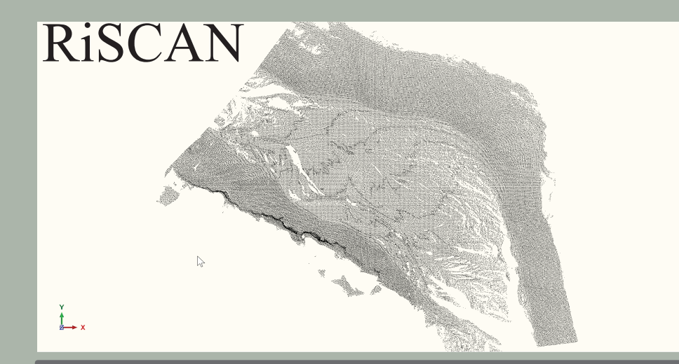
Figure 10: Visualization of a LiDAR point cloud in RiSCAN showing outline of Garwood Valley in Antarctica.
