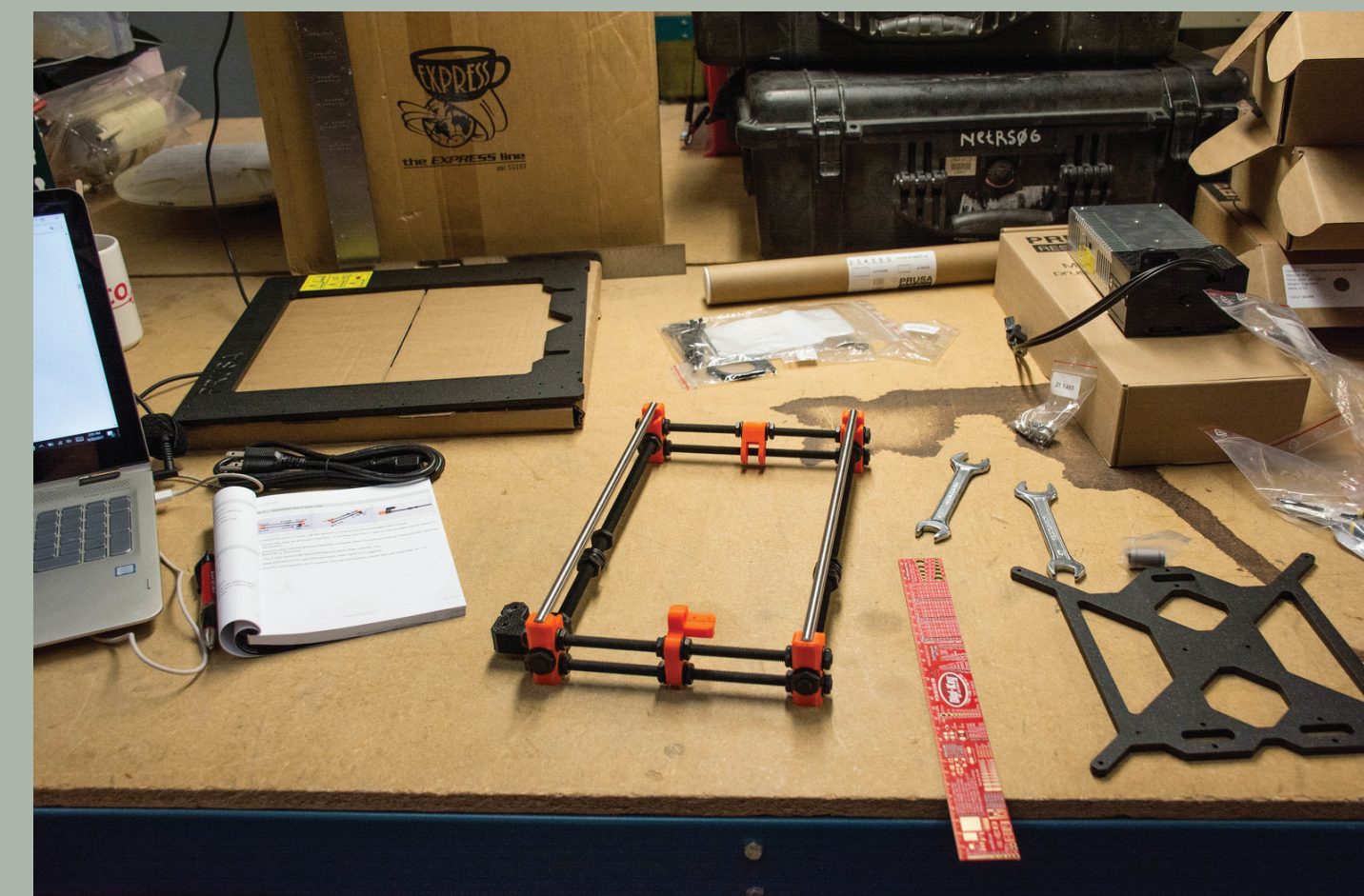
Figure 2: The Prusa i3 MK2 during assembly showing completed y-axis.
