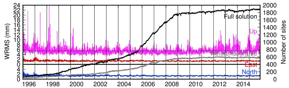
**Figure 3.** Evolution of the GAGE processed network over time. The weighted root-mean-square residual of the fit to the reference frame is shown in east (red), north (blue), and up (magenta) components, where the number of stations used to align the processed network to the reference frame is shown by the gray line. The total number of stations contained in the processed solution is shown by the black line.
