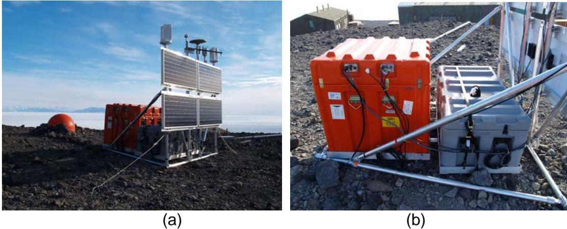
Figure 8. (a) Integrated GPS/seismic station MCMX at McMurdo.
