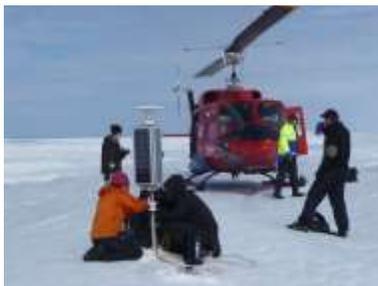
Figure 7 – Installation of winter-over GPS systems on the Greenland Fractures project. The systems are designed for rapid installation in high ablation areas, and further design upgrades are in progress including a method of “floating” the solar panel assembly on the ice surface to lower the center of gravity and improving the water tightness of the enclosures.
