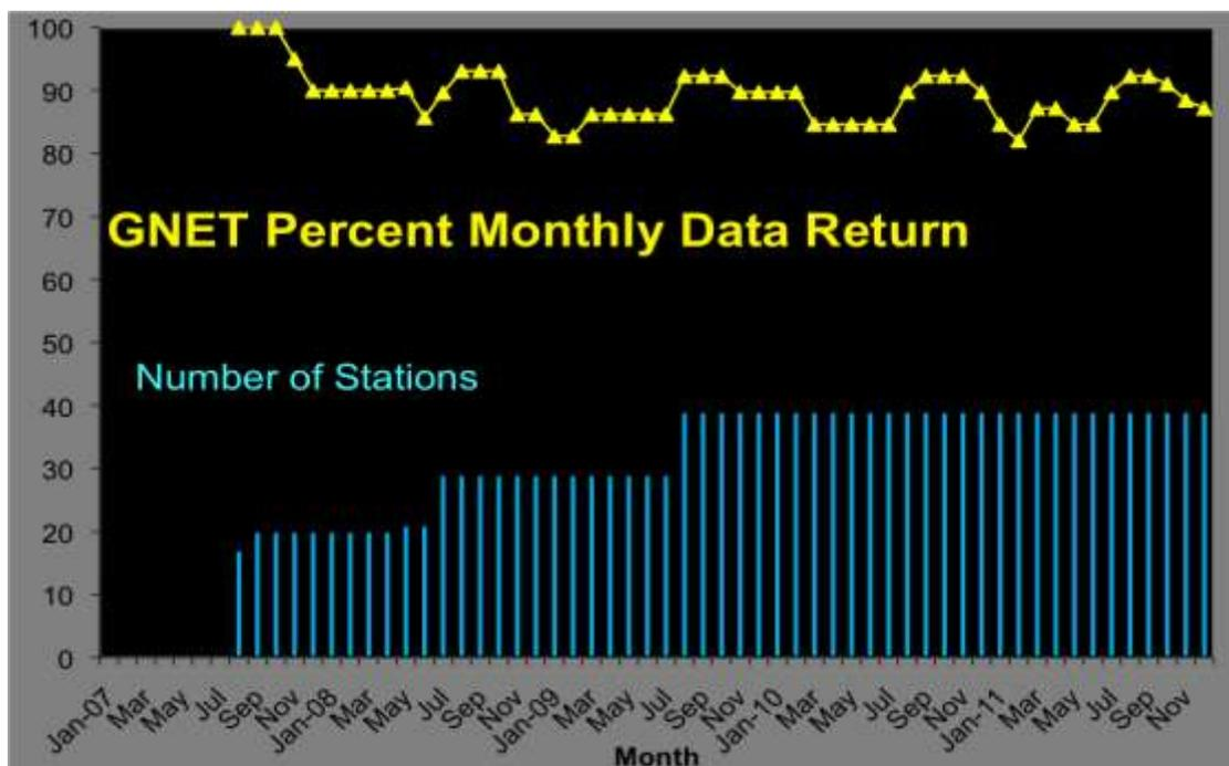
Figure 9 - GNET remote stations have achieved consistent 80-90% data return through 2011.
