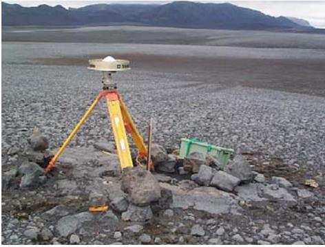
UNAVCO provided three receivers to collect an additional epoch of GPS measurements in order to capture the displacement field nearly two decades after a major rifting event at the spreading plate boundary in north Iceland between 1975 and 1985. The rifting episode resulted in up to 9 m of crustal widening, followed by a regional, post-spreading anelastic deformation transient involving up to a further 26 cm of crustal widening over the next decade, and decaying in amplitude with time.
