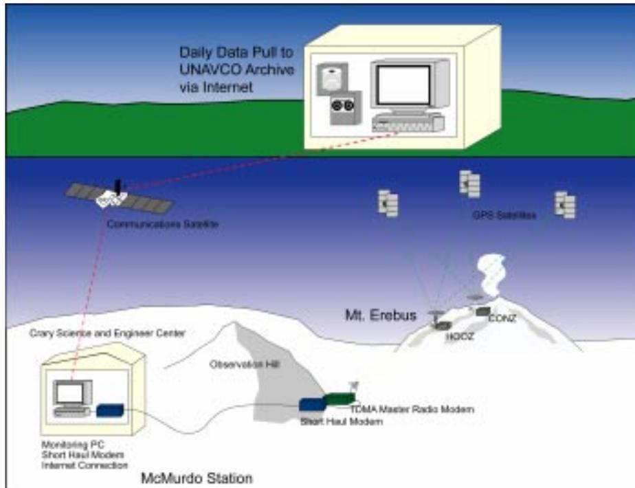
Figure 5 – Mount Erebus continuous GPS station diagram
