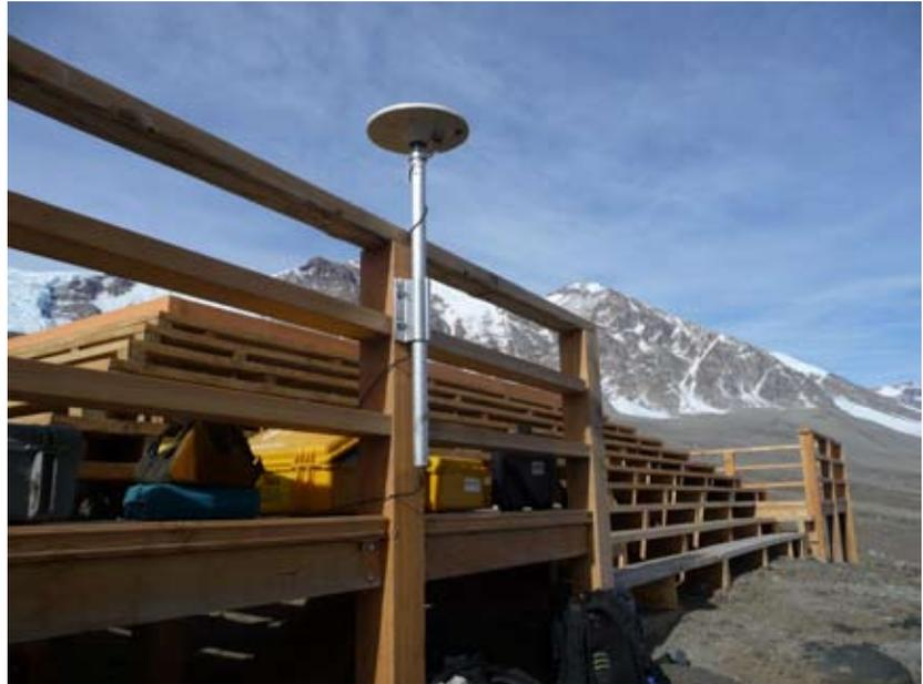
Figure 9: New benchmark BON1 installed on the helicopter pad at the Lake Bonney camp.
