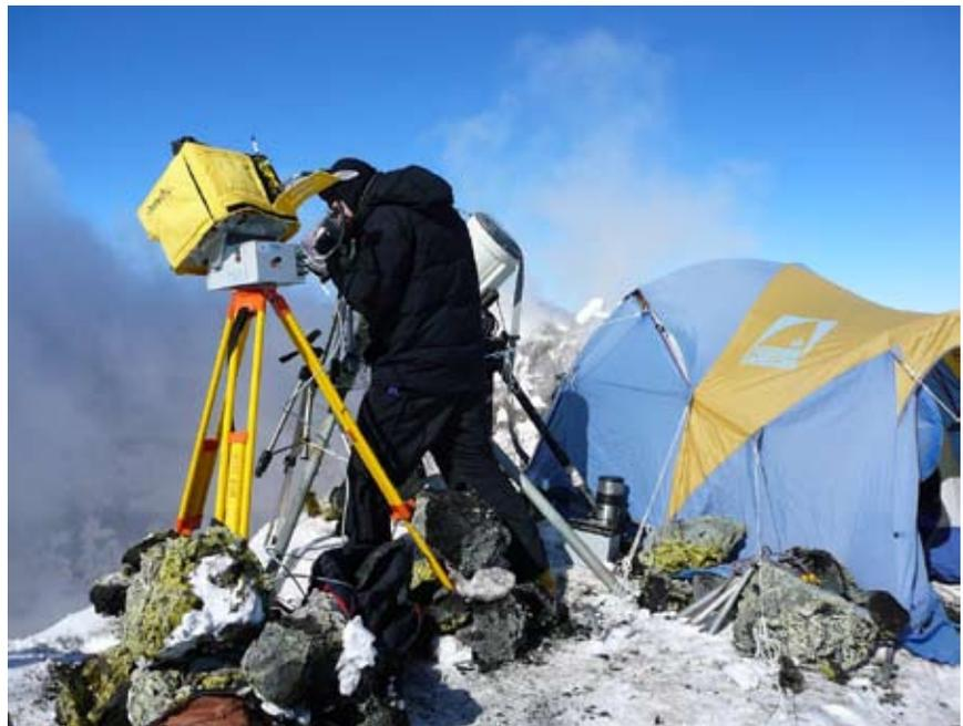
Figure 14: UNAVCO Ground Based LiDAR shown imaging the lava lake within the caldera of Mt Erebus, Dec 2009.
