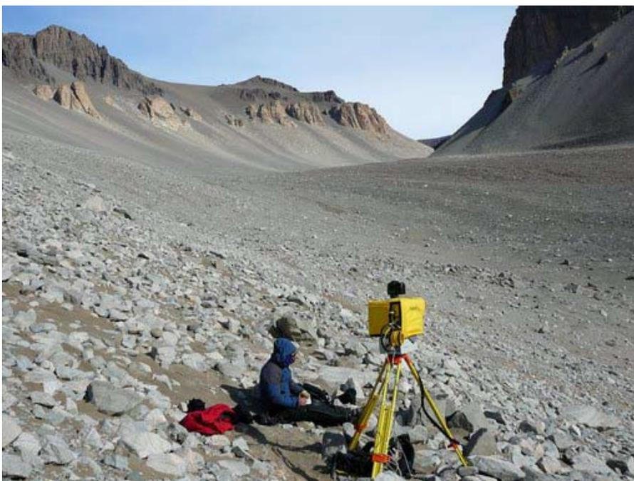
Figure 8: Hasnan Basagic using the Terrestrial Laser Scanner to image a rock glacier in the Dry Valleys.
