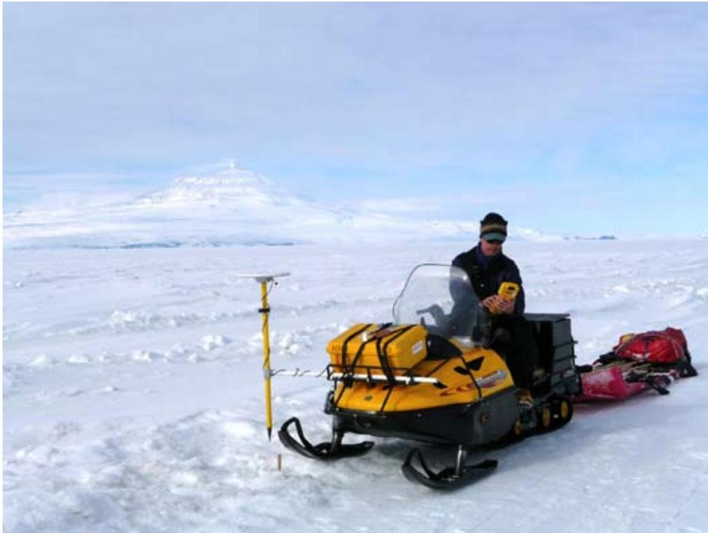
Figure 12: UNAVCO Field Engineer Joe Pettit operates the mobile GPS system used to measure a 50 km seismic shot line for G-049 at New Harbor, Nov 2008.
