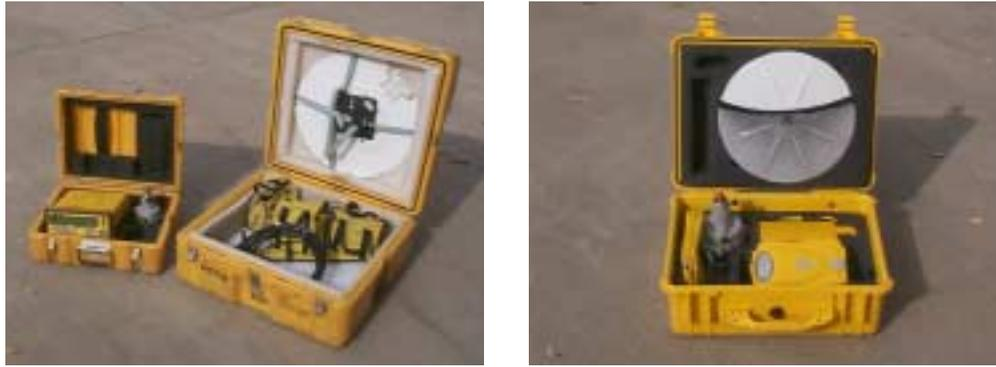
Figure 1. Traditional UNAVCO pool campaign system (left) vs. a modern GPS campaign system (right). The modern system is less than half the size and weight of the older UNAVCO pool systems.
