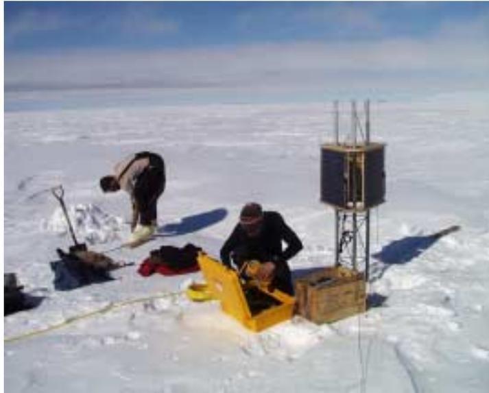
Figure 6. Installation of Trimble 5700 on iceberg C-16.
