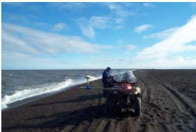
Figure 8. Kinematic GPS survey of Barrow coastline
