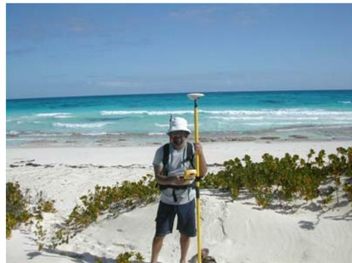
**Figure 3.** Engineering support section manager Jim Greenberg mapping marine stromatolites using real-time kinematic GPS at Highbourne Cay, Bahamas. This work was conducted for PI PamReid of U. Miami in support of a joint EAR/BIO initiative.
