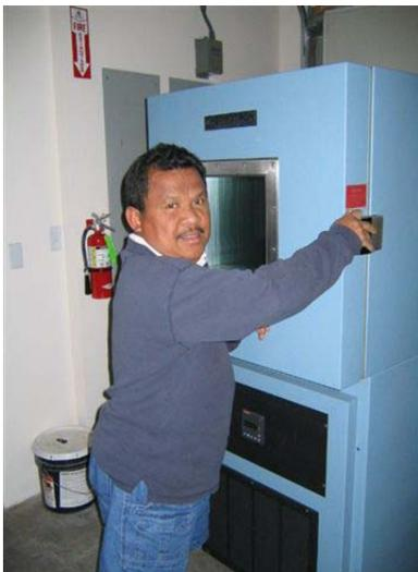
**Figure 5.** Equipment technician Effendi Sihombing demonstrating the Facility's new temperature test chamber, which was acquired to support highly controlled receiver data quality testing for various investigations.
