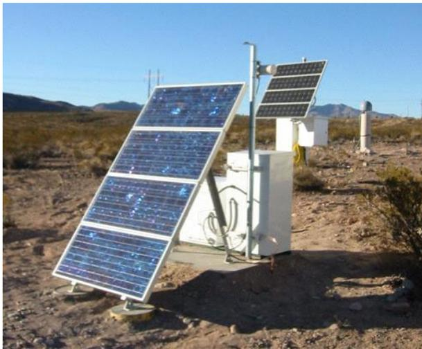
Figure 5. Joint GPS/Seismic site using VSAT telemetry at Socorro NM.
