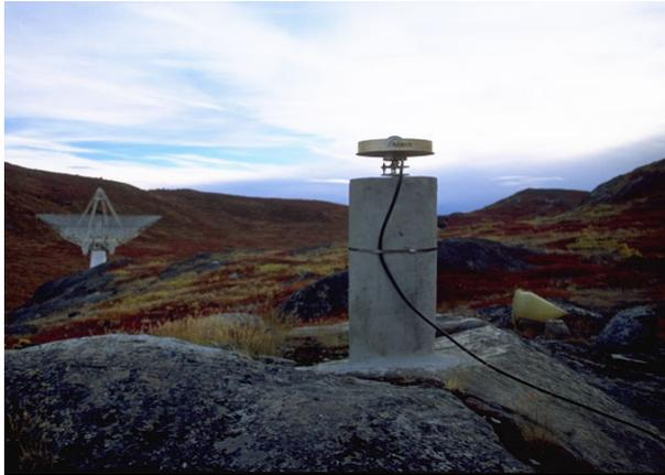
Figure 4. Site at Kellyville, Greenland upgraded to a GGN/RTNT capable site.
