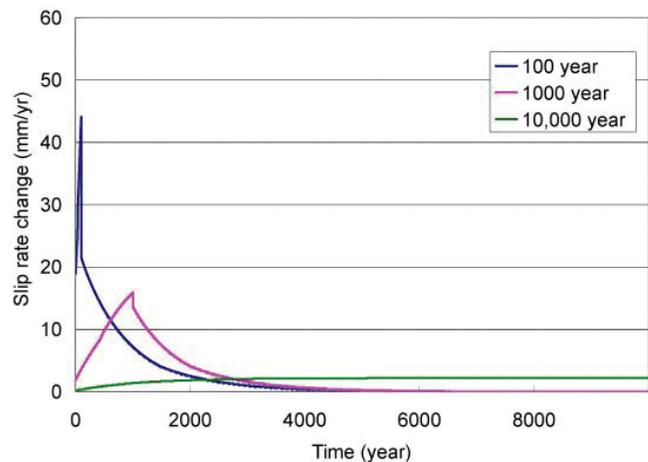
**Figure 1.** Predicted evolution of slip rates as 1 MPa  $\Delta\sigma_{RCFS}$  increase is accumulated over a period of 100 years, 1000 years, and 10,000 years, respectively. Slip rate decays afterwards. The peak of slip rate change is higher when the increase of the  $\Delta\sigma_{RCFS}$  is accomplished over a shorter period.
